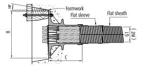
Notes: F range anchors are designed for minimum concrete strength fcmin= 22 MPa (on cylinder). The usual installation method is threading the strands into the ducts (flat sheaths) before concreting. However, if necessary, it is also possible to thread the strands after concreting the structure, on condition that special provisions are made.
